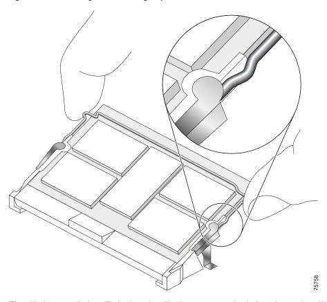
Figure 57 Inserting the Retaining Clip
